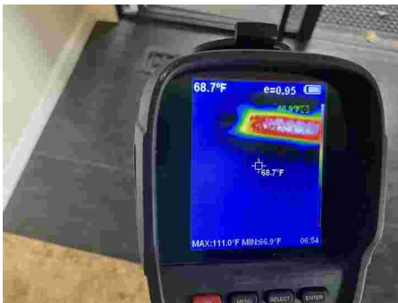
Register air out is 110deg.
