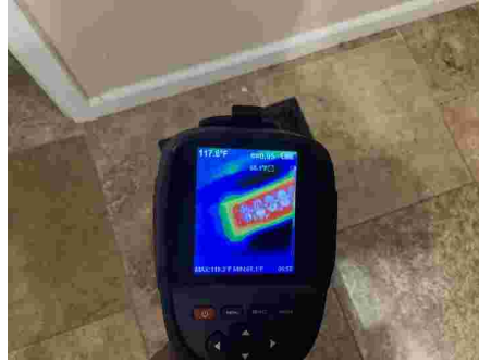
Heat at register 119deg
