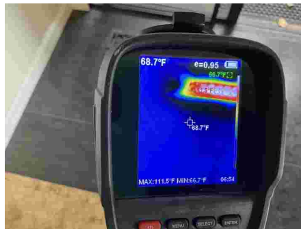
Heat at register 119deg
