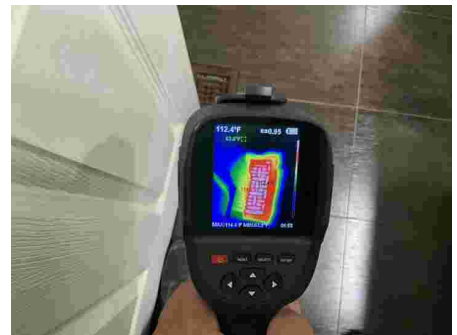
Register air out is 112deg.
